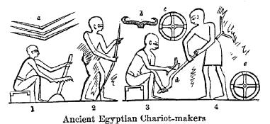
Fig. 1, Sawing out the Axle; 2, Preparing the bent pieces of Wood, a, b; 3, 4, Shaping the Pole, d; c, e, Wheels.
